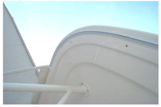
2. Once the  $5^{\circ}$  6" track is secure add a  $7^{\circ}$  6" pc to both ends. Track should extend around corner all the way to the arch Style support.
