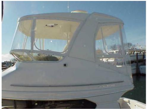
5. Slide all 8 panels into track and then zip all panels together. The front buttons are marked but not installed to allow for adjustment. Some special tools are needed to install these fasteners. Call 1(888) 245-0011 if you need help finding these tools.
