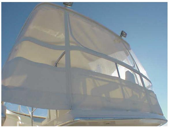
6. The aft section of the enclosure is secured with Bunji cords. Mark each location with a pad eye and secure with #8 x ¾" screws. The sides secured with LTD studs.
