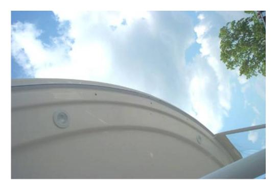
1. The track package consists of 9 pieces of track. The 5' 6" pc is for the front. Locate the center of the track on the center of hard top. Keep the track about a ½" from the feature on hardtop, as shown in picture Secure with the flex rail crews provided, screws should be installed every 6".
