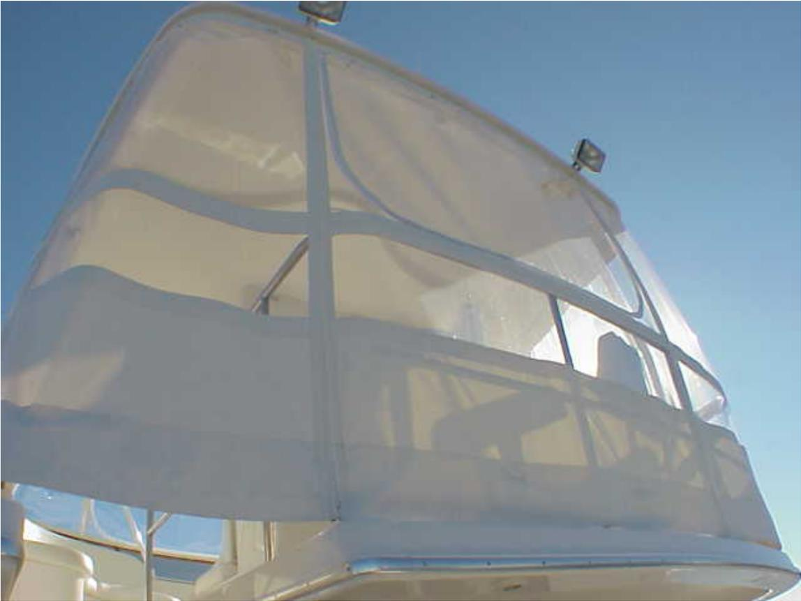
6. The aft section of the enclosure is secured with LTD studs. Install the side curtains first then work across back. Work from center out installing 1 or 2 studs at a time until completion. There are two 6" tracks not shown in these pictures. Locate the Velcro flaps on the side curtains. Install the tracks to hold the flaps in place. Caulk all holes and track.
