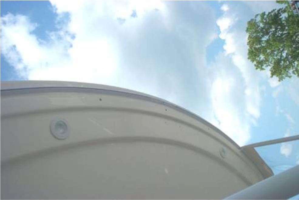
1. The track package consists of 11 pieces of track. The 5' 6" pc is for the front. Locate the center of the track on the center of hardtop. Keep the track about a 1/2" from the feature on hardtop, as shown in picture. Secure with the flex rail crews provided, screws should be installed every 6", caulk all holes before installing screws.
