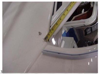
3. Begin installing the 47in track provided at the bottom base of the arch and work up so that the tracks over lap as shown in previous picture. Secure the track with the Flex Rail screws and bit provided. Repeat on opposite side.
