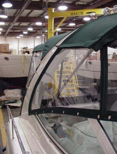
4. Remove the zip rope from the side panels and slide into the track. Zip the panels to the track and finish installing the remaining Lift the Dot studs provided.
