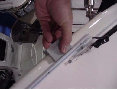
2. Use the track guide to draw a line at 1in from the front edge of the arch for the front side panels.
