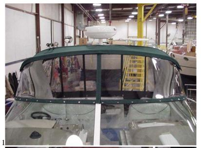
1. Zip all four panels to the top and to each other. Begin installing Lift the Dot windshield clips provided at the center of the windshield. Mark one button at a time and install. Mark out around the corner to the sides.
