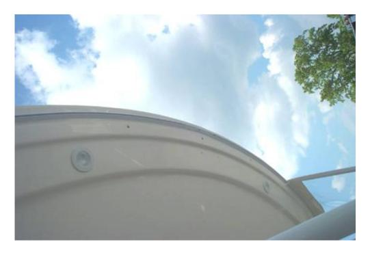
1. The track package consists of 11 pieces of track. The 5' 6" pc is for the front. Locate the center of the track on the center of hard top. Keep the track about a 1/2" from the feature on hardtop, as shown in picture Secure with the flex rail crews provided, screws should be installed every
