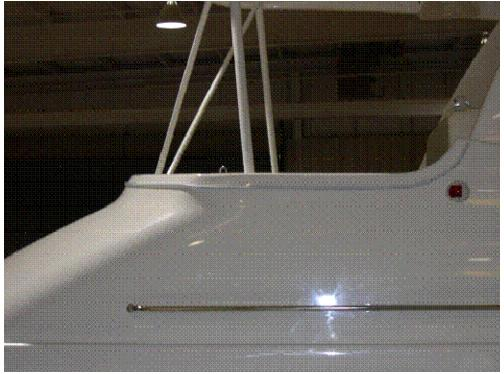
5. Slide all 8 panels into track and then zip all panels together. Scribe a line 2 ½" down from top of bridge (verify the line is ¼" down from the bottom of the enclosure panels). Install center of the 4' piece of flexrail to the center of the bridge (align top of the flexrail to the scribed line). Install 7' 6" pieces of flexrail on port and starboard sides of bridge (align top of flexrail to the scribed line).
