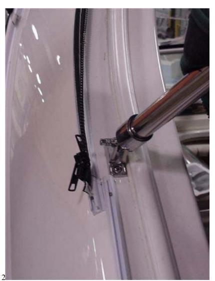
2. Begin installing the 63in track provided inside bimini track below top mount as shown in the picture. Work down the arch keeping the track tight to the mounts. Repeat on the opposite side. Remove the rope zipper from the side panels and slide into the track. Zip the panels down and install the remaining glove buttons on the bottom of each side.
