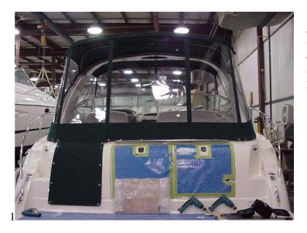
1. Zip all five panels to the top and to each other. Begin installing at the transom door with the buttons evenly spaced on each side of the opening. Work across the back and around the corners. Use Glove button studs provided.
